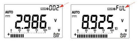
Figure 2-1 Manual logging display
