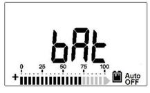
Figure 2-3 Battery capacity display
