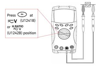
The frequency measurement is applicable for DC and AC current measurements.
