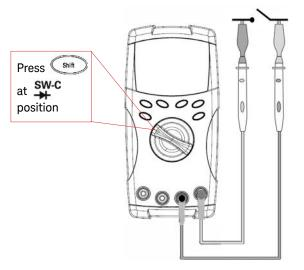
The switch counter is used to check the open/ close condition of a switch, relay or push button. The multimeter provides the time base of 10 and 100 seconds, or user-defined time base.
