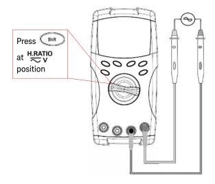
Harmonics ratio function indicates the deviation of non-sinusoidal to sinusoidal waveform from the range of 0% to 100%. A pure sinusoidal waveform without harmonics gives a value of 0.0%.
