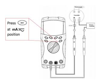
The % scale of 0 - 20 mA or 4 - 20 mA is selectable in setup mode. The mA% scale for 4-20 or 0-20 is indicated on primary display and the bar graph indicates the current value. The 25% scale readout represents DC 8 mA at 4 – 20mA, and DC 5 mA at 0 – 20mA.
